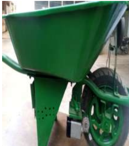
Fig.18. Electrically operated wheel barrow
