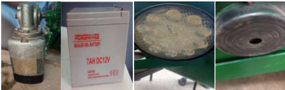
Fig.10. DC Shunt Motor Fig.11. Batteries Fig.12. LED headlamp Fig.13. Buzzer
